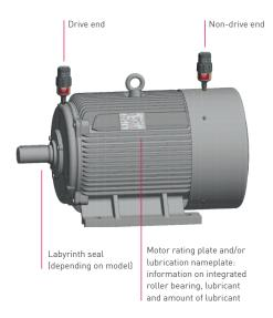
Lubrication points are located on the drive and non-drive end of electric motors. When relubricating, you must ensure that excess grease is discharged through the discharge openings, grease relief ports or grease traps. Bearings will overheat if grease cannot escape and I or if grease traps are filled up with used grease.
