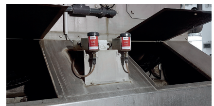
Bearing lubrication at excess sludge densifier
