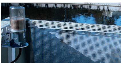
Lubrication of the slewing bearing
