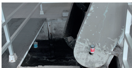
Lubrication of chain guide rollers
