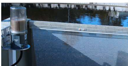
Lubrication of the slewing bearing
