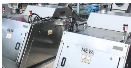
Lubrication of screen gears
