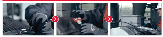
Clean the lubrication point, remove grease fitting
