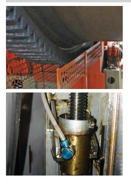
perma lubrication systems with suitable accessories for applying the lubricant to the gear surface guarantee effective relubrication. Permanent renewal of the lubricant film with subsequent lubricant distribution to additional gear wheel pairs helps to reduce wear in the long-term and increases gear wheel service life.
