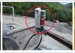
Lubrication of pillow block bearing on a conveyor
