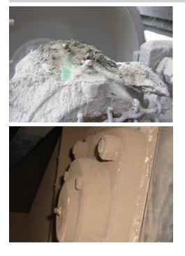
Service life and reliability of seals, roller and sliding bearings mainly depend on ambient conditions. Extreme operating conditions and the and contaminants in the bearing system lead to increased wear and to a shorter service life.
