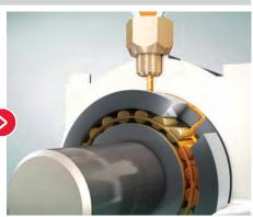
Once the system is activated fresh lubricant is discharged uniformly into the lubrication point.
