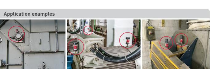
Flange bearing lubrication on bucket conveyor
