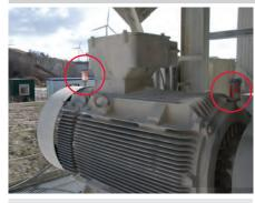
Motor lubrication on a vibrating screen
