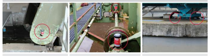
Roller bearing lubrication on a chain guide roller
