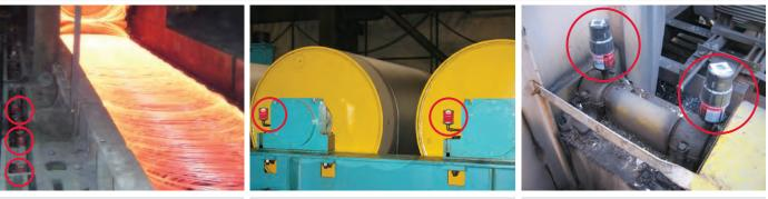
Drive chain lubrication (bolt stock conveyor)
