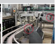
Chain lubrication on box transport system after packaging machine and full crate check
