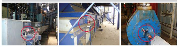
Flange bearing lubrication on a conveyor
