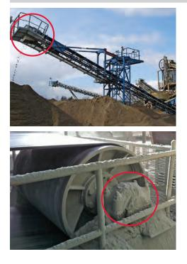
Large conveyors often extend over long distances and several levels and are **difficult to access**. Relubrication should ideally take place while the equipment is running. Many transfer points can only be lubricated with the help of catwalk grating or work platforms and are therefore often **neglected**. **Accident prevention** and **workplace safety** must be ensured at all times.
