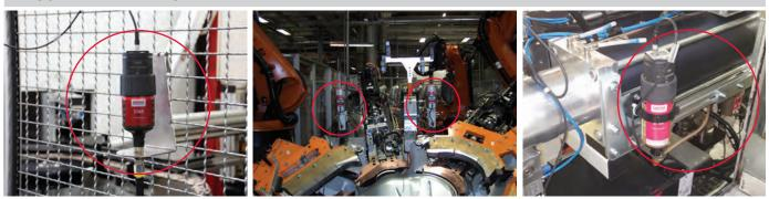
Automatic lubrication of a sliding guide
