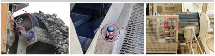
Lubrication of pillow block bearing on a conveyor
