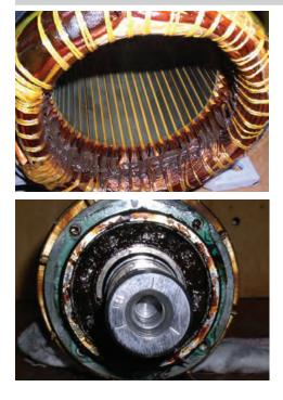
During manual lubrication, the grease is **applied in uneven amounts**. A large quantity of lubricant is introduced at one time. This leads to a temporary **over-lubrication of bearings**. Ignoring the recommended relubrication intervals leads to **lubrication starvation**.
