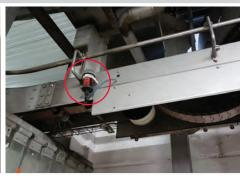
Chain lubrication on transport system box ejector
