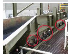
Bearing lubrication on the tree sorting system
