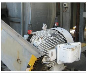
Industry: Application: Lubrication system: Installation solution: Mining Electric motor bearings perma STAR VARIO Direct mount
