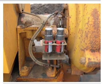
Industry: Application: Lubrication system: Installation solution: Mining Slurry pump perma STAR VARIO Remote beam clamp mount
