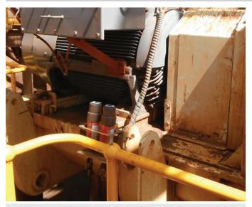
Industry: Application: Lubrication system: Installation solution: Mining Electric motor bearings perma STAR VARIO Remote beam clamp mount
