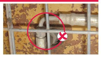
ightarrow When using reducing adaptors with fine threads such as 6 mm metric or 1/4" UNF select stainless steel to avoid breakage
