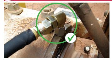
perma STAR VARIO lubrication systems have a G1/4 male thread at the grease outlet. Where reducers, elbows or extensions are required to simplify installation it is important to adhere to the following guidelines:
