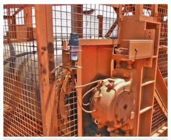
Industry: Application: Lubrication system: Installation solution: Iron ore mining Conveyor bearing / seal (hybrid solution) perma STAR VARIO Remote cage hanger mount perma Lubrication Systems
