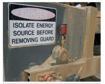
Industry: Application: Lubrication system: Installation solution: Quarry Conveyor bearings perma FLEX Direct mount
