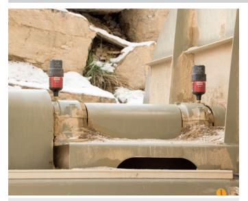
Industry: Application: Lubrication system: Installation solution: Quarry Fan / blower bearings perma STAR VARIO Direct mount
