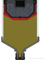
Activation cap with integrated gas generator (PA GF)
