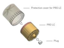
Place the PRO LC inside the protection cover and remove the plug of the PRO LC.
