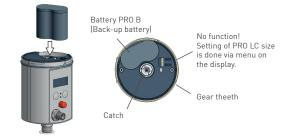
Insert the battery PRO B into the drive unit (according to the direction of the arrow on the label).
