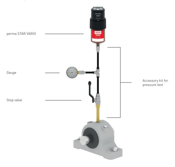
For pressure testing please use perma STAR VARIO with Accessory kit for pressure test (101480).
