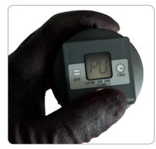
10. If counter pressure doesn't decrease you need to either select a different lubricant or a different lubrication system. Please ask perma to assist you in this matter.
