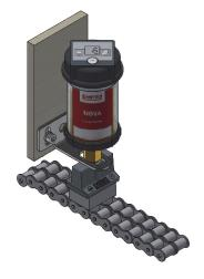
In order to extend the service life of chains, lubricant must be specifically applied to the wear points within the gaps of inner and outer lugs, as well as rollers, bushes, and pins.
