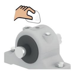
2. Remove grease nipple or plug screw of connecting thread and check thread size.
