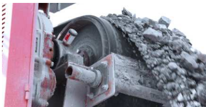
Lubrication of pillow block bearing on a conveyor
