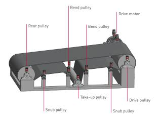
Pillow block housings with spherical roller bearings are mainly used for drive and bend pulleys.
