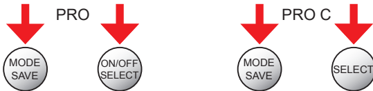
figure 11 For a manual initialization, press and hold down both buttons of the lubricator simultaneously.
