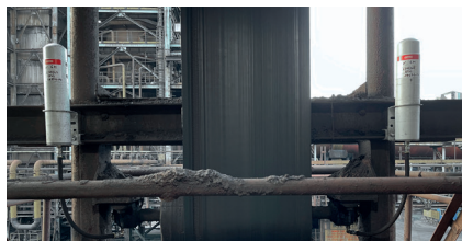
Lubrication on a conveyor (tension pulley)
