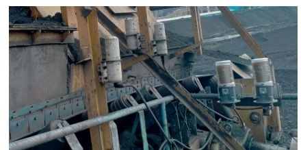
Lubrication on a bucket excavator
