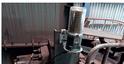
Lubrication on a conveyor (drive pulley)
