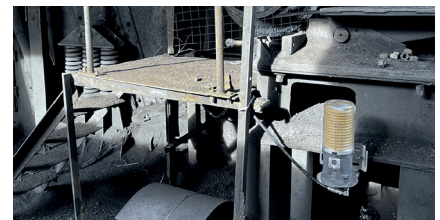
Lubrication on a vibrating screen
