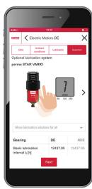
The software will recommend the **most suitable lubrication system**, the ideal lubricant and the right discharge period.
