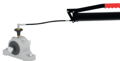
For direct mounting: Prefill lube-point and any connecting parts (use the same grease that is contained in the lubrication system)
