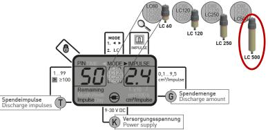
Figure 4: New display in IMPULSE operating mode with four LC variables, discharge impulses [T], discharge amount [G] and power supply [K].
